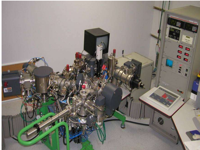
Figure 6: Image of Cameca 6f SIMS instrument (magnetic sector)
