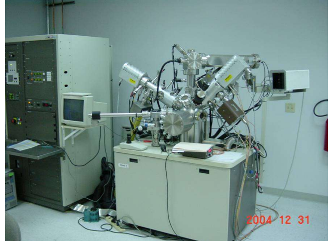
Figure 7: Image of PHI Adept 1010 SIMS instrument (quadrupole)
