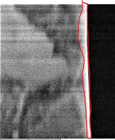
*Figure 12: SEM imagery of  $(\text{ZrO}_2)_{0.93} \cdot (\text{Y}_2\text{O}_3)_{0.07}$  on Polished Zr at 100 mJ*
