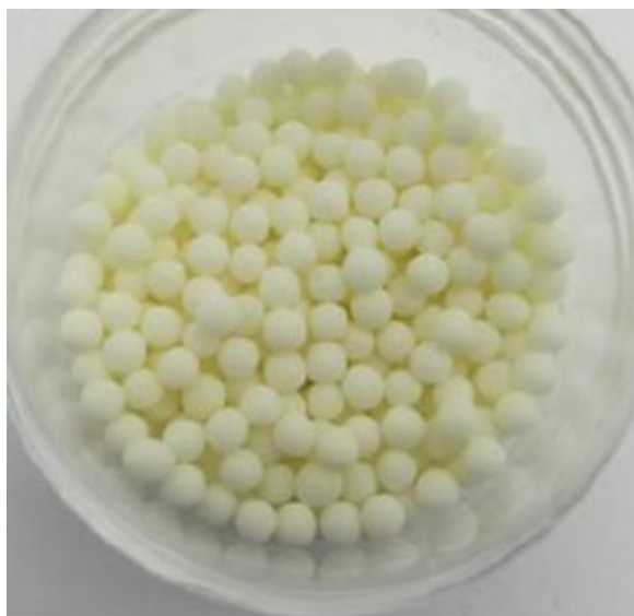
Figure 6. \text{In}_2\text{O}_3 impregnated YSZ beads. (photo by Daniel Piatek)
