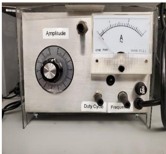
Figure 9. Power supply and voltage signal. (photo by Daniel Piatek)
