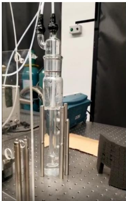
Figure 8. Bubbler used to introduce humidity to CO 2 gas line. (photo by Daniel Piatek)
