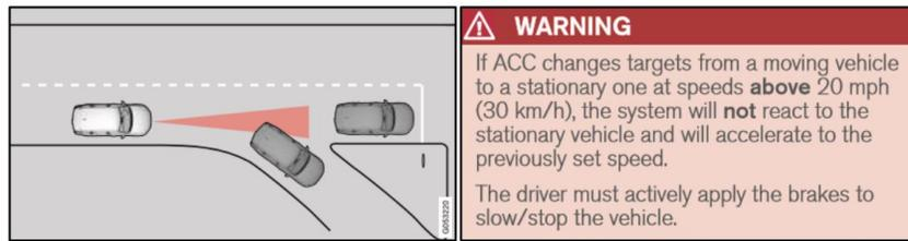
Figure 3: ACC Cut-Out Scenario Warning, 2016 Volvo XC-90 Owner's Manual<sup>32</sup>
