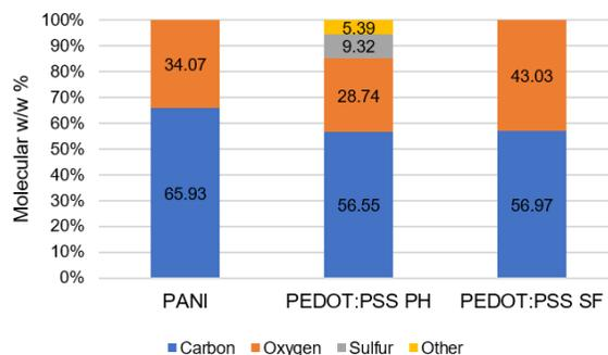
**Figure 8. Energy dispersive x-ray spectroscopy of polymer samples.**
