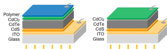
**Figure 3. Layered cross-section of polymer (left) and control (right) cells.**
